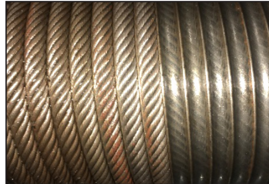
Wire rope with Chesterton 601 Chain Drive and Bushing Lubrication and 715 Spraflex Gold applied.
