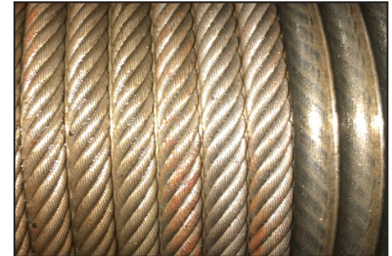
After a month of application wire ropes are still free from dirt and dust build up.
